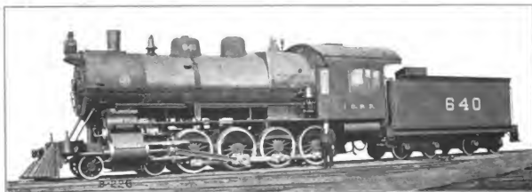
Fig. 74. Twelve-Wheel (4-8-0) Locomotive. Built by the American Locomotive Co. for the Illinois Central. Cylinders 23 in. x 30 in., Working Steam Pressure 210 lbs. per sq. in., Heating Surface 3,494 sq. in., Diameter of Drivers 57 in., Weight on Drivers 193,200 lbs., Total Weight 232,200 lbs.
